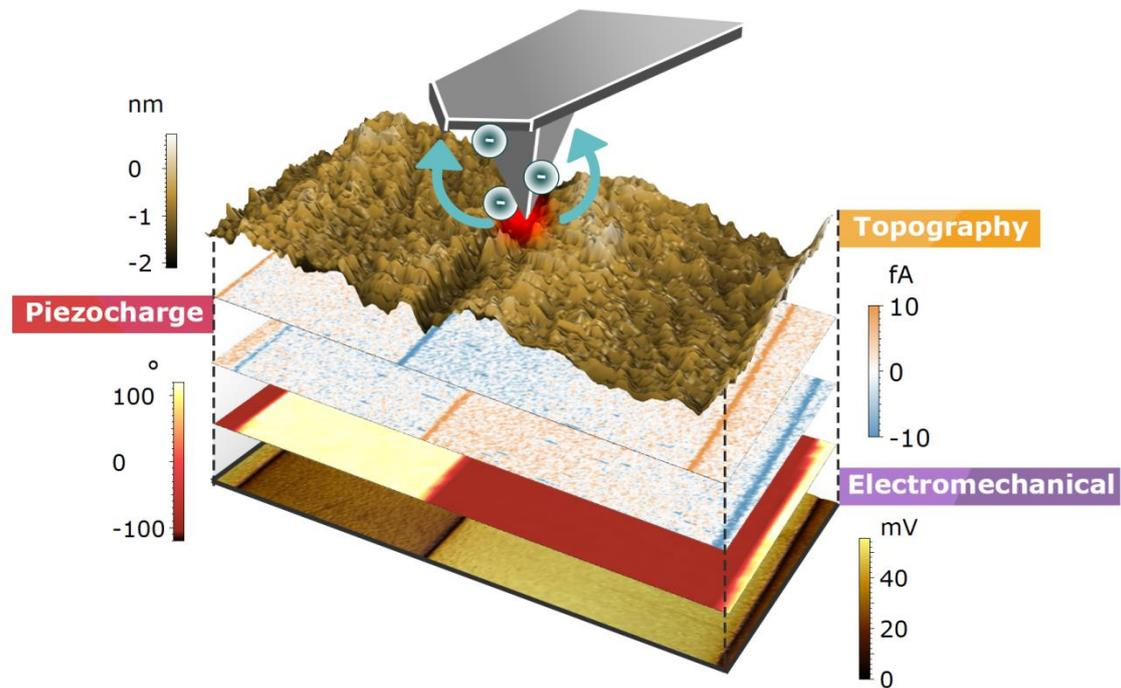
**Figure:** 3D composition in which the tip that scans the surface along with the rest of the properties of the material is represented, such as the topography, the generation of charge (fA), and its electromechanical response. Image size is 30x15 micrometers.
